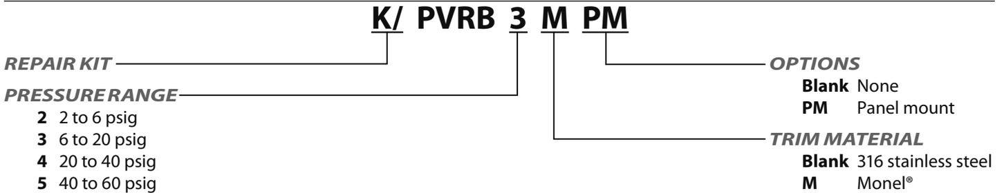
Note: if this regulator is to be used in oxygen service, specify "GENERAL OXYGEN SERVICE" when ordering or furnish the factory a copy of the special requirements.
