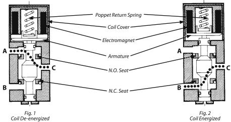
**The De-energized Position** With the valve in a de-energized position and pressure applied to Port B, the valve operates as a 3-way, 2-position, normally closed valve. In this position a flow pattern from Port A to Port C is established (figure 1). Pressure can be applied to either port. The forces affecting the poppet are on the normally closed seat resulting from the poppet return spring.
