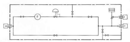
The P42-433 is a Type 1-1 Configuration manifold designed for low pressure, high flow system use. Applications include torpedo launching, pneumatic tube systems, pressurization of aircraft, etc. The manifold body is naval brass with stainless steel trim. The operating pressure of the manifold is 135 psi. Service is air.
