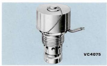
This normally closed cartridge type solenoid valve has an operating pressure of 0 to 2000 psi. The service is air or nitrogen. The VC-4075 is of continuous duty in design and operates at voltages from 18 to 28 VDC. The valve has a  $C_V$  factor of 0.5. The body of the valve is anodized aluminum with stainless steel trim.
