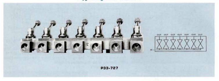
The P33-727 is an oxygen regulator manifold valve that controls the flow from a single inlet source by means of six plug shutoff valves. The valve was designed for use in experimental deep diving vehicles and inspection of offshore drilling sites. Low pressure (0 to 10 psi) supplies oxygen, helium, and nitrogen. The body of the manifold is made from monel for protection against corrosion.
