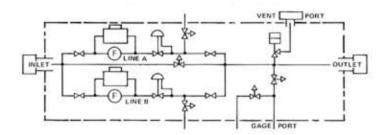
This dual circuit oxygen service manifold was designed to comply to the requirements of Configuration 2-1. The body of the P39-433 is monel with stainless steel trim. The flow rate of the unit is 58 SCFM.
