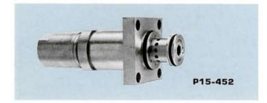
This pneumatic relief valve is supplied for use in special breathing systems aboard Salvage and Rescue Ships. The body of the valve is 303 Stainless Steel. The full flow pressure is 2150-SCFM of gaseous nitrogen and oxygen.
