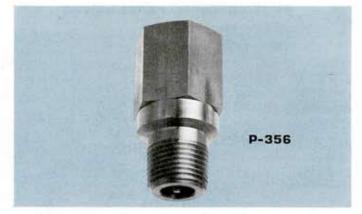
This brass bodied check valve is designed for use as a vital component in military aircraft fuel systems. The P356 has an operating pressure of 85 psi and a maxiumum cracking pressure of 5.0 psi. The valve will function in any position in the system. Aircraft fuel with octane ratings of 115 to 145 are compatible with the valve.
