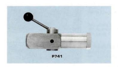
A combination manual shutoff and check valve is utilized as a vacuum system component. The valve operates at a pressure of 0 to 15 psi. The valve body is of commercial brass. The cracking pressure of the check valve is 0.5 to 1.0 psi. Air is used as a fluid media.
