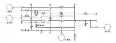
This Sulphur Hexiflouride Insulating Manifold contains 5 different types of valves. A total of 17 components comprise the complete manifold. The system was designed for a manufacturer of heavy duty electrical systems. The manifold controls both the flow and the pressurization of the insulating gas in both the high and low pressure side of the system. The manifold is available in aluminum. The operating pressure of the manifold is 300 psi.
