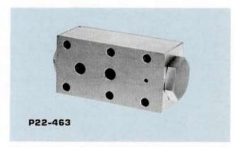
This double check valve is for line mounting or subplate (sandwich) mounting applications that utilize NFPA porting that match NFPA 4-way valves. The P22-463 is a standard-off-the-shelf item. The valve is available in Aluminum or Ductile Iron. The rated pressure of the valve is 3000 psi with a flow of 8.5 GPM.
