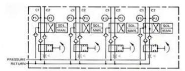
This hydraulic manifold was designed for use on large naval vessels that required automatic and remote operation of the main ballast valves. Each manifold unit contains 4 to 5 repetitive valve circuits. Each circuit contains check valves and relief valves as system components. The body of the manifold is carbon steel with a black oxide finish. The P34-433 has an operating pressure of 2000 psi and is compatible with MIL-H-19457 Type oil.
