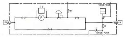
The P40-433 conforms to the requirements of Configuration 1-1. The flow rate of the manifold is 5 to 80 SCFM. The inlet and outlet fittings are 1" and 3/4". The body is naval brass with stainless steel trim. Service is air or gaseous nitrogen.
