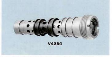
This spool type valve is designed for use as a component for manifolds that are part of tank hydraulic systems using MIL-H-5606 and MIL-H-6083 hydraulic fluids. The V4284 has an operating pressure of 3000 psig and a flow rate of 10.0 GPM. The exterior of the valve is hard coated aluminum, while the interior is stainless steel.
