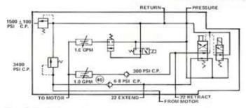
The P25-433 is a high pressure hydraulic manifold with an operating pressure of 3000 psi. It was designed to function as a component in the fire control system of a missile launching tank program for the U.S. Army. The manifold was an integral part of the magazine indexing system. It was engineered to use both MIL-H-5606 an MIL-H-8063 Hydraulic oils. The manifold body is aluminum.
