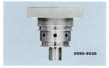
The 2990-9530 is a cartridge type high pressure breathing gas regulator for Deep Diving systems. The body of the valve is made of 303 Stainless Steel. The inlet pressures of the valve ranges from 850 to 3800 psig with flow rates from 40 to 3000 SCFM. Service is gaseous oxygen and helium.
