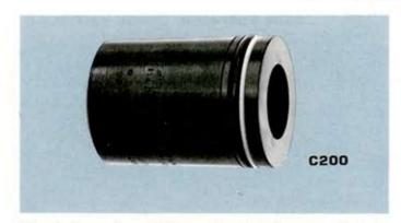
This leakproof cartridge check valve provides a precise, compact, non-leaking valve for use as an integral component in manifolds designed for pneumatic and hydraulic systems. The C200 operates at a pressure of 0 to 6000 psi. It offers positive sealing at any differential pressure. The valve is available in aluminum, steel, and stainless steel. The C200 is compatible with virtually all liquids and gases.
