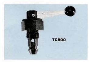
The TC900 is a cartridge type shutoff valve. The valve has an operating pressure of 0 to 6000 psi. The valve is fabricated from steel. The stem and seat design of the valve permits rapid actuation of the handle with a minimum of opening and closing shock to the system. The TC900 is a standard catalog item and is compatible with most fluid media.
