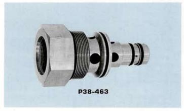
This cartridge mounted pilot operated check valve is designed for use as a component utilized in critical applications that control cylinder drift. The P38-463 is also used to lock in position variable pitch propellers on large ships. Service is hydraulic fluid.
