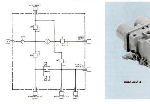
The P43-433 is a solenoid operated manifold designed to function as a control for oxygen breathing systems in military aircraft. The operating pressure of the manifold is 110 to 2250 psi. The manifold contains five separate components: Solenoid Valve, Check Valve, two Relief Valves, and a single Filter assembly. The body of the unit is anodized aluminum.
