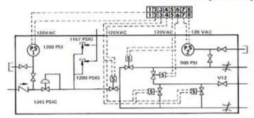
This complete system controls the operation of a brake system plus controlling the helium pressure supply to an inflatable seal. The manifold contains 17 individual components housed in a carbon steel body. All functional components are of stainless steel. The manifold operates at a pressure of 1400 psi and utilizes helium as a service fluid.
