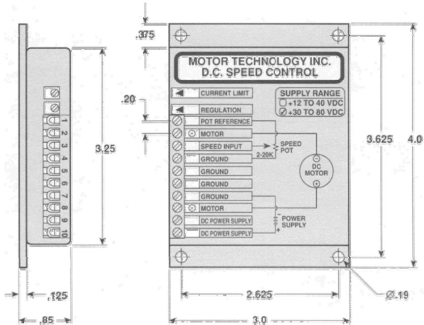
\*The customer is responsible for providing the remaining circuit components (i.e., potentiometer, fuses and computer control).
